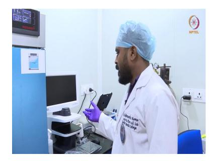
Apart from that, and this one is inverted fluorescence microscope from these we could be able to see the live cells with the help of fluorescent dyes like Alexa Fluor, Dapi and Cy 3. So, usually that fluorescent microscope has three different color range, one is red and green and blue. With the help of these different dyes we could be able to track the particular cells morphology and their internal organs organelles and the nucleus also ok.
