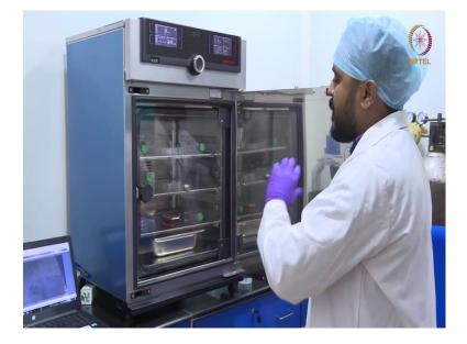
First one, is like for a in vitro cell culture the main important thing is like is CO 2 incubator, why it is very important is like our human body have maintained the same constant temperature and constant oxygen supply and constant carbon dioxide supplies it will be there for inhalation exhalation.
