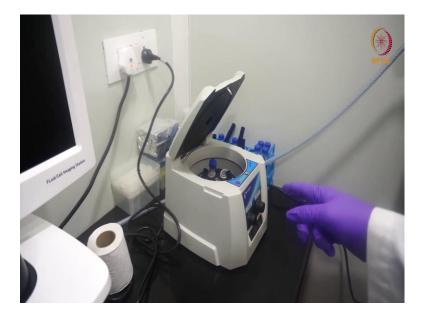
And centrifuge is also very important thing to separate and isolate and culturing and further subculturing the cell lines ok.
