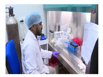
So, this is the working platform this is the in vitro cell culture working platform so, called biosafety cabinet. Our biosafety cabinet is class 2 b 2. So, here the mechanism means that the outside air should not enter inside and inside air should be circulated and then it will go towards the outlet that.
