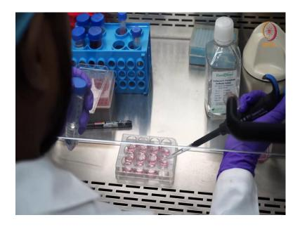
So, again one more wash to discard the leftover dye and with the help of phosphate buffer saline, after discard the fluorescent dye. Now, I am going to place it in the inverted fluorescent microscope to absorb the cells and whether it has a pick the dye or not and with the help of fluorescent microscope.
