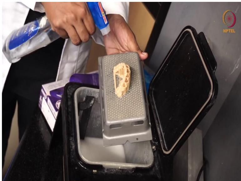
So, use isopropyl alcohol first to clear off the dripping resin and this is the tank in which the isopropyl alcohol is stored.
