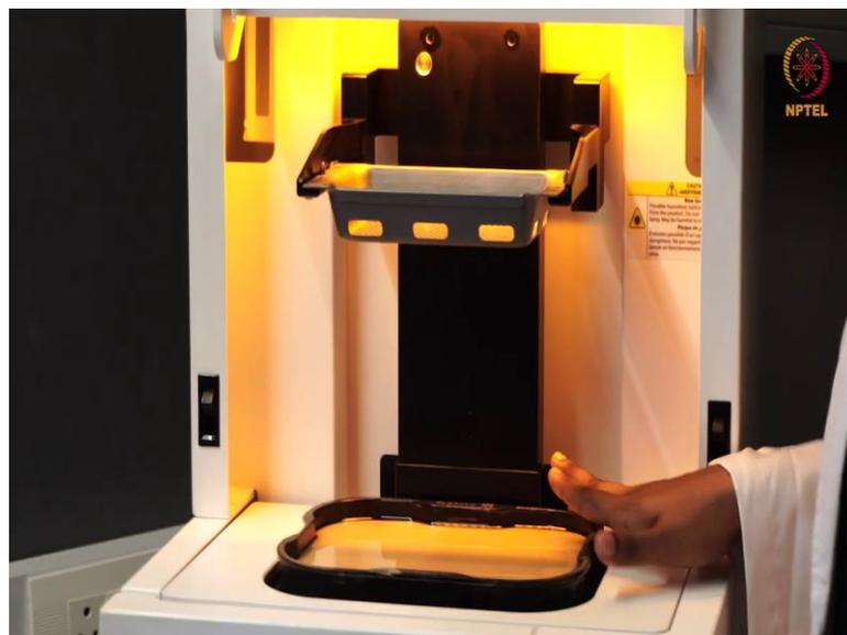
So, before starting we should ensure that the resin platform is full with resin and the printing bed is clean. Having known this basic about this digital light processing printer. Now, let us focus on the SLA printer that is the stereo lithography technique printer. This printer is an example for SLA technology printer.
