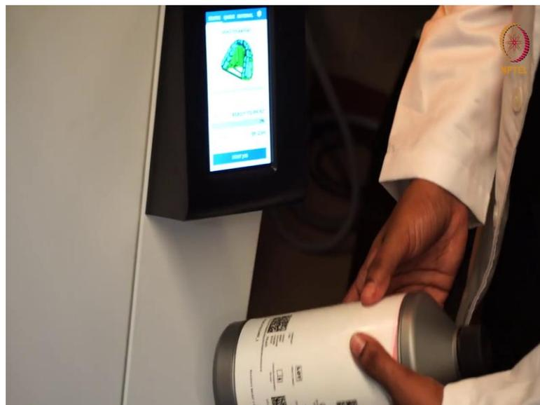
And then, the resin which we are using has to be scanned here. This is the foolproof system, because any outdated or expired resin will not be accepted by the printer. So, once the resin is identified next we have to double check whether the platform is clean and the resin is stirred and the printer is stable.
