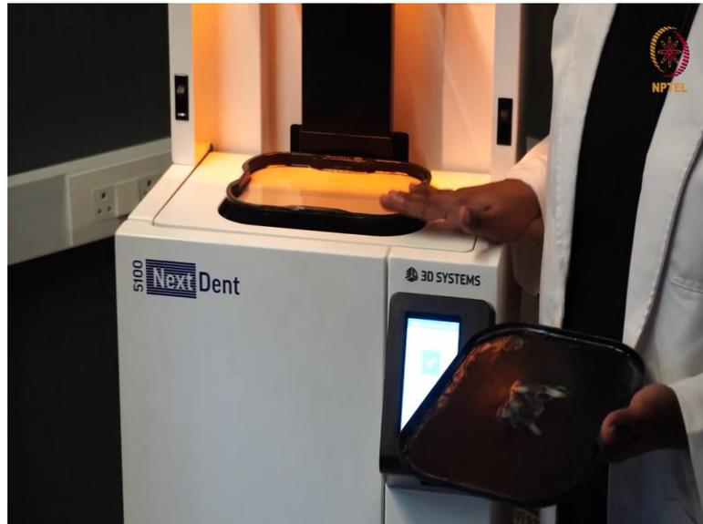
Next you have the resin. So, this is the photo polymerizing resin. So, you can see that this is the resin tank in which the resins are stored. So, there are different resins for example, model resin which was used for laboratory purposes, surgical resins which are used for printing of body parts, then we also have flexible resins with in which we can print flexible structures. So, we have a lot of other resins also available for the printing.
