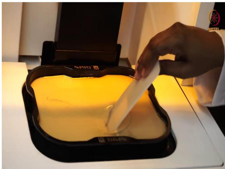
Now, you can see that the resin is in layers. So, I have to ensure it is thoroughly mixed before starting the print. So, all these factors will affect the quality of the print. So, now you can see that we have achieved a smooth texture of the photo polymerizing resin. So, this means that we are ready to print.
