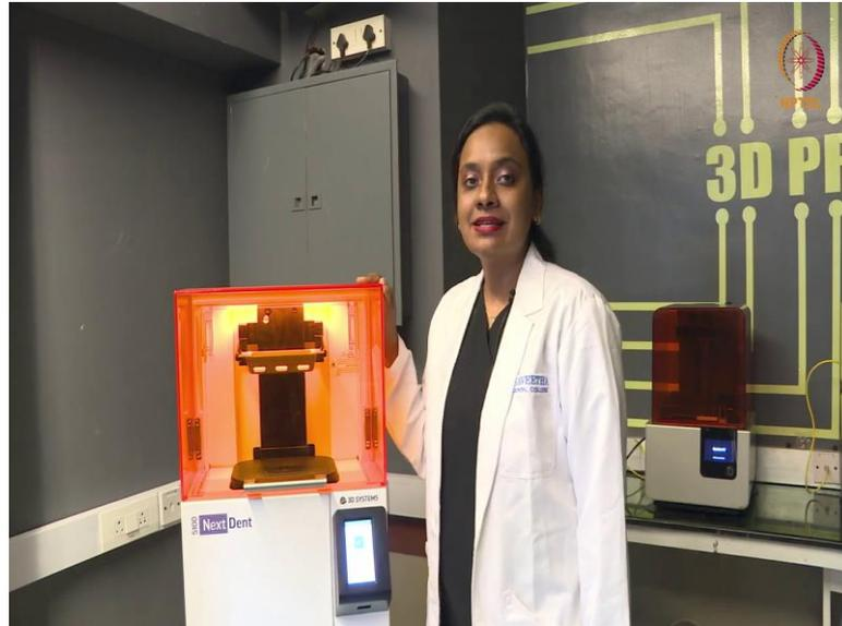
Now, the printer next to me is an example of digital light processing technology. So, what does this printer have? First let us know, what are all the constituent parts of a printer?
