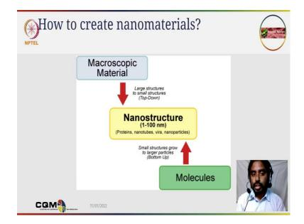
So, for the fabrication of nanomaterial's, two things can be two approaches can be used; one is top-down approach, another one is bottom-up approach, right. So, top-down is you have a bigger material, you are crushing them into smaller size and then you are making a nanomaterial, right. So, that is called as top-down approach.
