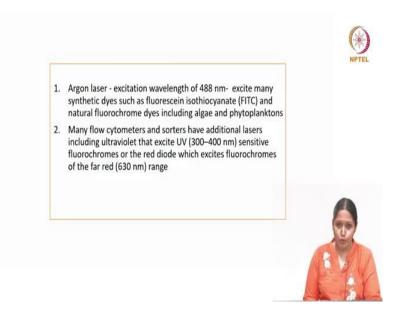
So, we use different type of lasers in flow cytometer, one such laser is Argon laser. Argon laser it has got an excitation wavelength of 488 nanometer, argon laser it will excite many synthetic dyes such as fluorescein isothiocyanate and natural fluorochrome dyes such as algae as well as phytoplanktons. And many flow cytometers and sorters have an additional laser which includes ultraviolet rate that excite UV at the wavelength of 300 to 400 nanometer.
