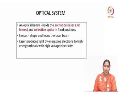
So, just now we have discussed about one of the major components of a flow cytometer that is fluidic system, next moving on to the optical system. So, optical system mainly it consists of an optical bench that holds the excitation optics as well as the collection optics. So, what is the excitation optics that we use in flow cytometer? It includes laser and lenses. So, laser and lenses are the excitation optics that we use in flow cytometer and then comes the collection optics.
