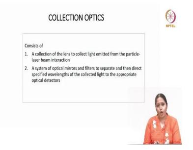
So, as I mentioned optical system consists of excitation optics and collection optics, Excitation optics mainly include lasers as well as lenses. Now, let us see what are the collection optics. So, collection optics consist of collection of lenses that are used to collect the light emitted from the particle laser beam interaction. So, after the particle and the laser beam interaction light will come right, that light will be collected by the collection optics.
