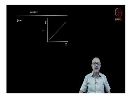
For example, Georg Ohm. Let me draw a line here. Ohm was trying to find out the relationship between the voltage across a piece of wire and the current passing through that piece of wire. So, voltage and the current. He made an arrangement by which the voltage can be varied in steps and for each value of the voltage, he measured the value of the current and he found that when voltage increases the current also increases.
