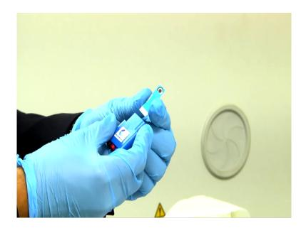
See, this is commercially available 3 electrode system painted shape you know. So, this center side is the working electrode, this semicircle black one is a counter electrode and a small this semicircle is the reference electrode. So, this is commercially available. Similar kind of electrode we can design for different kind of disease diagnosis. So, not only like the glucose different kind of other analyte can be detected that I taught it in the class.
