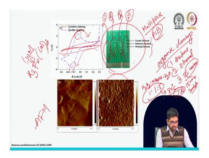
Let us show you this all the technology like PCB, this is the another design of the PCB that I showed you last class, that PCB I already used like three electrodes. Here, this is a multiplex PCB right, multiplex PCB. Why I am saying this is the multiplex? Because, you can see 1, 2, 3, 4, 4 see unit there.
