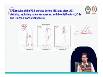
Then, after the AFM study if you wanted to check that, yes, your surface really clean or not, let us check the XPS, photo electron spectroscopy, X-ray Photoelectron Spectroscopy, that I showed all that in last class. Today, again I am summarizing here, you can see that the BC means just Before Cleaning, AC means After Cleaning. See, the gold peak, see this is the before cleaning is very less, but after cleaning it is very high.
