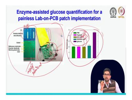
And, this is the actual structures that actually I wanted to show you, the structures of the PCB that we integrated some microfluidics. So, at the very first slides I showed you that microfluidics can be integrated some different different way. In this case, I am showing you that microfluidics can be just this another layer. So, here is two different type of the microfluidics we use 1 and 2, two pattern we use.
