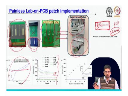
Let us show you how we can implement a patch right. So, I wanted to develop a very simple patch like bandaid right. And, here this patch we will use a PCB, but this PCB will be flexible PCB, flexible. Why I am saying flexible? That, these PCB substrate should be a flexible substrate, on that flexible substrate you have to print these all the these all the working reference counter electrode you can print, that can be done easily ok.
