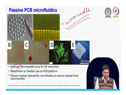
So, for this development of this patch based biosensor so, you have to collect the interstitial fluid, as I told you need some microfluidic like this. So, on this microfluidic there is some (Refer Time: 27:30) So, here your all the interstitial fluid means you can inject and it will go through. But, when it will be the real patch then it will collect, it will put on your skin it will collect the interstitial fluid, where you need some very small needle.
