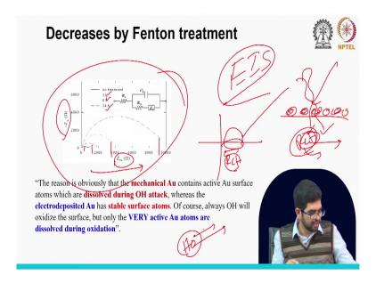
So, this decreased activity also we measure with the help of impedance spectroscopy the EIS, Electrochemical Impedance Spectroscopy. I think you remember last time I taught you like if this is the x-axis we are measuring the impedance of real value and y-axis we are measuring the imaginary value. So, and you can remember I think, right. So, like this impedance this semicircle this R this is the R ct charge transfer resistance. So, based on this value we can measure the electron transfer rate.
