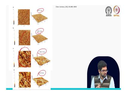
So, here is the whole images you see when your surface not polished just before polished 1.7 nanometre and, in that case, just sonications 1.6 nanometre not that much change and this is the surface just after polishing this is the AFM Atomic Force Micrograph images 13.8 nanometre and then after sonications it become 8.4 nanometre. So, we can clearly see the changes.
