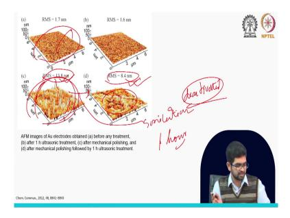
So, first we investigated the surface roughness. As I told you in the Fenton treatment that before the Fenton reagent treatment the surface become very see very rough after the mechanical polishing you can see the surface roughness 13.8 and then after the sonications when the sonicate sonication for like 1 hour if you go for the 1 hour sonication you see surface becomes smoother and roughness become 8.4. So, it was 13.8 now become 8.4 nanometre.
