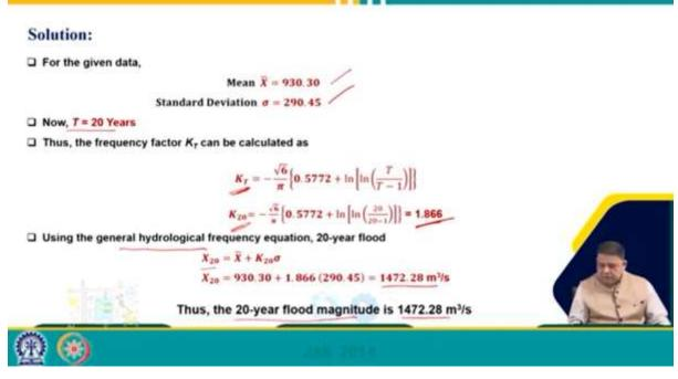
The 20-year flood magnitude is 1472.28 cubic meters per second. So, that is how we can use the frequency factor method for finding out or fitting the frequency analysis.
