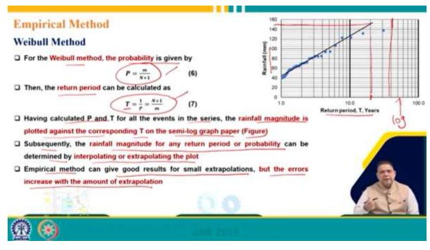
For the Weibull method, the probability is given by P = M/N + 1. The return period, T, is the inverse of P, or equivalently, P is the inverse of T. Therefore, the return period, T, can be calculated as N + 1/M.
