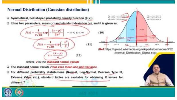
Now, to give you an idea, the normal distribution, also known as the Gaussian distribution, is a symmetrical bell-shaped probability density function, denoted by f(x). It is a two-parameter model characterized by its mean and standard deviation. Mathematically, it is expressed as follows
