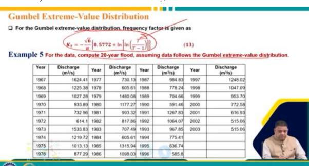
Another example is to compute the 20-year flood assuming the data follows the Gumbel distribution. Given the data and the calculated mean and standard deviation, we calculate the value  $k \cdot x_t$  for t = 20 using the Gumbel extreme value distribution equation. This yields a k value of 1.866, and using the general hydrologic frequency equation, we find  $x_{20}$  to be 1472.28 cubic meter per second.
