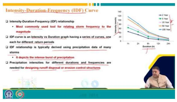
Now, let us discuss the intensity-duration-frequency curve once we have talked about frequency. The intensity-duration-frequency curve is the most commonly used tool for relating the storm frequency to the magnitude, and it is an intensity versus duration graph with a series of curves, one for each different return period. Here, you can see that we have intensity on the y-axis and duration on the x-axis, and these are curves for different recurrence intervals or frequencies.
