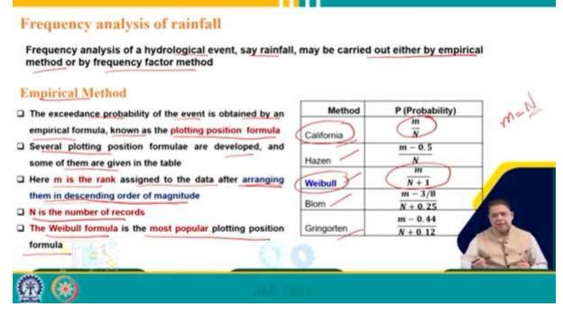
Now, let's talk about the frequency analysis of rainfall and hydrologic events. Frequency analysis can be conducted either through empirical methods or by frequency factor methods. In the frequency factor method, there are two possible ways of analysing frequency.
