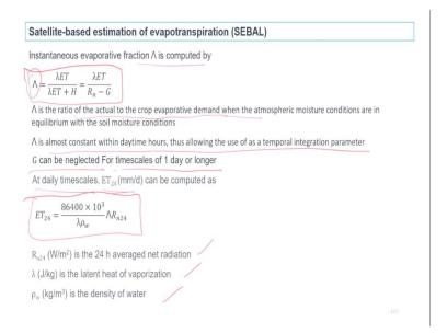
So, SEBAL model, in fact, allow you to understand the different extremes of weather events like humidity, temperature. Because ultimately, you are going to also calculate the evapotranspiration. So, the instantaneous evaporative fraction is computed using this equation.
