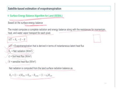
Now, satellite-based estimation of evapotranspiration. This is another utilization of satellite-based technology. Surface Energy Balance Algorithm for Land, this is what we call as SEBAL. This is actually used and it is based on the surface energy balance theory. The model, it computes a complete radiation and energy balance along with the resistance for momentum, heat, water vapor transport for each pixel, for each pixel. So, this is the equation that is used for this
