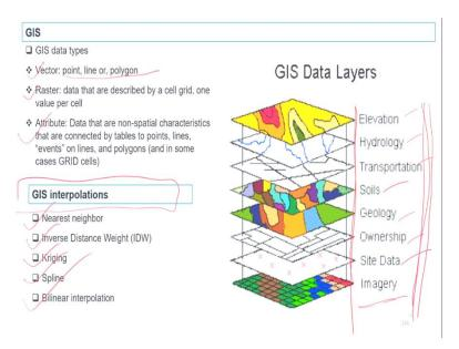
So, if you look at the data types that GIS tool uses they are basically vector and raster data. Vector data are in the form of point, line or polygon. Raster data that are describing by cell grid, one value per cell. Then you have attribute data that are non-spatial characteristics that are connected by tables to points, lines or events and polygons in some cases also grid cells.
