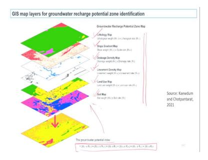
GIS map layers for groundwater recharge is very interesting and lot of work has been carried out across the world. So, especially for groundwater recharge if somebody wants to study then you can see that you need various layers, means various level, various type of information. Lithology map is one, slope gradient map, drainage density map, lineament density map, land use map and soil map.
