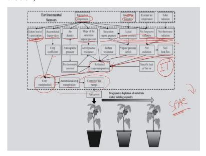
Now, this particular site is actually shows the different kind of sensors which can be used for agricultural farming systems applications and specially water applications. Now, if you see the different environmental parameters which are important for a plant growth; for those kinds of parameters sensors are actually developed. Now, what are the things that we need, temperature one of the most important parameter, humidity and these two parameter can easily be sensed through some sensors.
