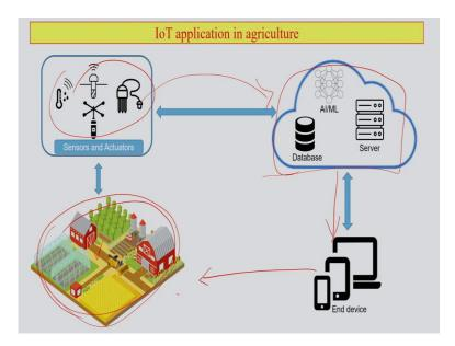
So, otherwise as a technology it has potential in the field of natural resource management. So, this is a very simple of schematic diagram that how IOT can be applied in the field of agriculture and natural resource management. So, this is your field and you can have various kind of sensor into this field and suppose that you are an owner and having only two three persons to look after the entire area, then I think that IOT application would be a very effective one.
