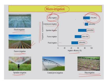
Now drip irrigation, as I said that it gives the highest amount of efficiency. So, it is enough that we spend a little time on this particular technology which is known as drip irrigation. Now drip irrigation or drip system, it has various techniques and instrumentations involved with that. So, it has pressure guage, venturi system, sand filter, screen filter, hydro cyclone filter, non return valve, by pass valve and then from here you are pumping out the water.
