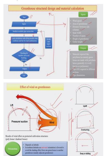
Now look at that, how greenhouse structural design, and also the associated various calculation with regard to the material can be carried out for preparing greenhouse gases under precision agriculture. Now, to start with, there are two important aspect or parameters that are associated with the greenhouse gas structural design those are inputs and what are the corresponding outputs.
