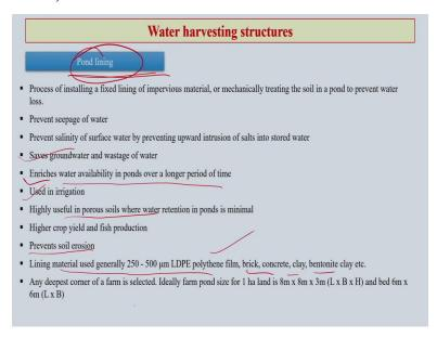
So, this is how you see that different water harvesting structures it helps. Pond lining is also important in case of water harvesting structures in the rural area. So, the lining of pond is critical to avoid the erosion of the soil and also you allow the water to get stored in that particular pond for a longer time.
