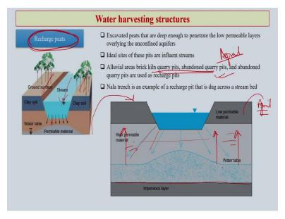
The second type of in our water harvesting structure at the community level comes recharge peats. Now, recharge peats are made through excavations which are deep enough to penetrate even the low permeable layers overlying the unconfined aquifers. So, before the aquifers even if you have a low permeable layer, this recharge peats will allow you to take that water even into aquifer crossing these semi permeable or less permeable layers.
