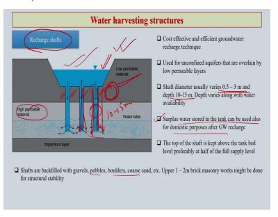
So, next comes the recharge shafts, now as you see in this picture is a little different than the previous two. Here, again, we have the water body or the stream here, here you allow through some channels the water to go into the water table directly and here you can have in between also the high permeable material here and low permeable material here.
