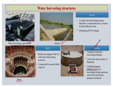
These days many kinds of new materials are coming for water harvesting structures; geotextile, geosynthetics, these are some of the things which are coming increasingly in case of water harvesting structures. Anicut, we are already using in many cases in southern part and also in the western part. These are basically small water harvesting missionary dam which are normally constructed across a stream and the water is largely used for irrigation and also for drinking purposes.
