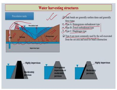
So, this is a very simple water harvesting structures, but has very good effect on recharging groundwater. So, how actually, it works; percolation tanks. So, as you see that this is the picture it can explain you about the technicalities of percolation tank. So, this is the water body the tank you have, you can have a small bund here in case this water level rises and should not go there.
