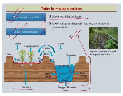
Modification of a village tanks and on-farm water management, these are again very common in our Indian condition. This modification of village tanks, on-farm water management normally carried out through lining of pond, desilting of pond, then tank and farm ponds, percolation
