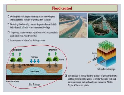
Then comes these days biomitigation is coming heavily and that how actually you can utilize different kinds of plant species and also how you can actually create a bio drainage system so that the drainage network can work in an appropriate manner. You can do it either improving the existing channel capacity or creating new channels.
