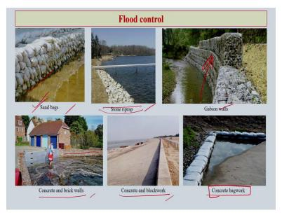
Sandbag, this you have seen many places; stone riprap also are being used along the side of the river, then gabion walls also are here used if you anticipate that your water level could actually rise with the rainy season; then concrete and brick walls are often used and these are seen largely in the developed countries and sometime also you can see it in some coastal regions of India in a different format.
