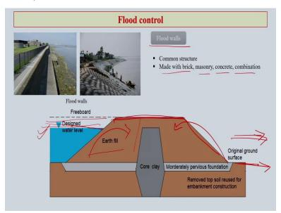
Now, there are various ways that flood can be managed; one is flood walls, which is one of the most common way common structure that we see in and around us, normally made with brick, masonry, concrete or combination of all those things, even some time sand bags are also being used.
