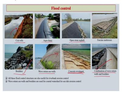
One step ahead if we want to go with the technology options, we have coir rolls also, which can be used as you see here, the coirs that you get that can be made roll and then you can across the slope pack it so that if in case of rising of water, it can actually get soaked there in this coir and then it actually also allows to the soil to get the appropriate amount of moisture. So, this helps in both ways.
