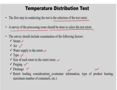
So the temperature distribution test is nothing but to see which is the coldest point in the container itself or whether my container receives the process temperature uniformly, right. So that is what we wanted to do temperature distribution test so my container everywhere the temperature is distributed uniformly or not. So that is what we are meant by temperature distribution test.
