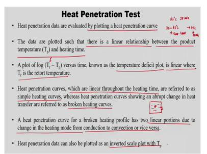
So the heat penetration data are evaluated by plotting a heat penetration curve. So the data are plotted in such way that there is a linear relationship between the product, temperature and the heating time. So right, for example, if I am telling the 63 degrees centigrade for 30 minutes so first I need to heat my product temperature to 30 to 63 degrees centigrade so this involves the time temperature combination, right.
