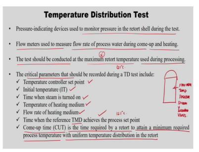
And also you need to remember the earlier classes. So we also told right, so the retort will have flow meters, then temperature detectors then pressure then for steam the bleeders, vents etc. So I also need to ensure the pressure indicating devices should be used to monitor the pressure in the retort shell and
