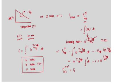
So the Z value is nothing but same concept but is at x-axis so you have a temperature which is in degree centigrade. So in y-axis you have log DT values. So the same linear log linear relationship, so the slope is nothing but minus 1 upon Z right. So from this I can find out my Z value which is which will be in degree centigrade. In the previous graph so what you get here is DT which is in time unit either minute or second, okay.
