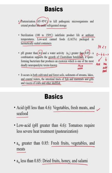
So the basics are, actually the thermal processing can be done in two ways. One is the pasteurization, so which accounts the temperature in between between 65 to 95 degree to kill pathogenic organisms which is nothing but a disease causing microorganism and extend the product lifetime and a refrigerated storage. So whenever you pasteurize, so you need to store it in a refrigerated condition, but whereas the sterilization is done in the temperature range between
