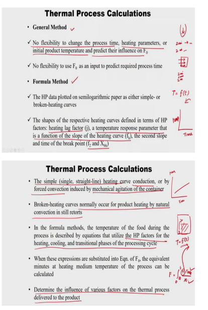
And thermal process calculation as we discussed already. General method, general method is nothing but a experimental method, so here there is no flexibility to change the process time and heating parameters. For example, if I am I am taking in the glass tube some of the food particles and initial known microbial counts then what I will be doing is for each two minute I will be taking out my sample each two minute and calculate my microorganisms level.
