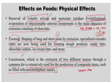
The removal of volatile solvent and monomer residues, volatile solvent and monomer residues so this is one example would be the fiber spinning so the melt extrusion comes from the polymer processing only, so I am taking the polymer example so you got you suit PAN a polyacrylonitrile so this is dissolved with a DMSO solvent dimethyl sulphoxide so after the extrusion so the fiber whatever you get out of the extruder will have DMSO solvent in it.
