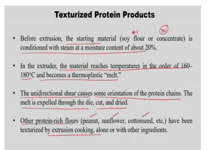
Before extrusion the starting material which is nothing but a soy flour concentrate or may be a 40 percentage or 70 percentage based on which one you need at the final product is conditioned with steam at a moisture content about 20 percentage. So that is the pretreatment, first is the starting material is conditioned with a steam at a moisture content about 20 percentage. In the extruder the material reaches the temperatures in the order of 160 to 180 and becomes thermoplastic melt.
