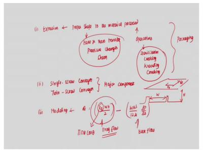
So in yesterday's lecture what we have seen is, the process of extrusion so that means a this is nothing but gives the proper shape to the material, proper shape to the material processed. The mechanism involved are heat and mass transfer, so pressure changes and shear and this is not only gives the proper shape there are lot many operations are, operations so which are what I remember is sterilization can be done, sterilization cooking can be done.
