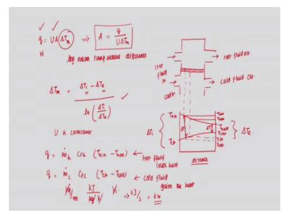
So, this is where the concept of log means temperature difference has come so LMTD. So if you remember in all the calculations we have used q is equal to UA Del Tm, all right? So this is nothing but log mean temperature difference, so what does it mean? So, it means so I am putting this as a wall. So, here is your hot fluid in, so here is your hot fluid out, so cold fluid in, I am taking co-current flow and a cold flow it out, okay?
