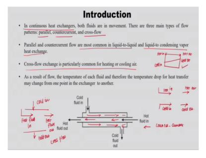
So, in introduction in continuous heat exchangers both the fluids are in movement, right? So mostly the heat exchanger we use for continuous flow. In continuous a heat exchanger both fluids are in moment. There are three main types of flow patterns, one is parallel counter current and cross flow. So, one example would be this one, so this is a counter current,
