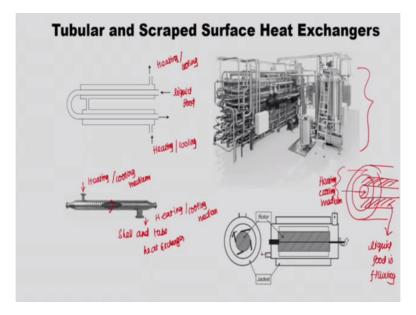
So, here is what your double pipe heat exchanger so which is nothing but a tubular heat exchanger. So your hot fluid goes in here or you can say your liquid food material is inside the tube liquid food. So, your heat medium or heating medium in terms of heating or cooling medium in terms of cooling flows this side, heating or cooling medium, okay.
