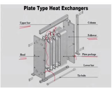
So, here we see, so this is the plate type heat exchangers looks like. So this is your upper bar so, this is your head plate, head plate in the sense header and this is the follower, right? So in between the header and follower your plates were arranged. So, as I said so here your hot fluid is flowing and here your hot fluid is flowing, here your hot fluid is flowing, so there is a mechanism which transfers this hard fluid to here and so here your cold fluid is flowing, right.
