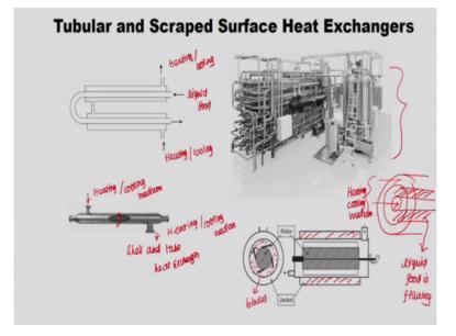
So, the scrap the surface heat exchangers, so which has a, they consist of a jacketed cylinder equipped with the central dasher with scrapping blades, so that is right here. Here, so this is your jacket so in the middle you have a rotor right so the rotor has blades. So this is the side view, so this is blades, so this is a rotor, so at this place your liquid food with the high amount of solid particles stays there okay.
