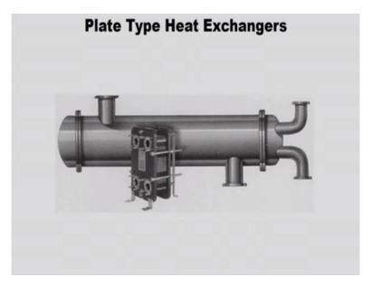
And if you compare your shell-and-tube module and plate module this is the way it looks like so in that way it is very compact compared to shell and tube heat exchanger.
