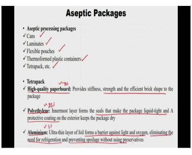
So the package is normally aseptic process packages, cans, laminates, flexible pouches and plastic containers, tetra packs all are aseptic packages. The tetra packs contains three components mainly, one is high quality paper board, so which gives the strength and brick shape to the packaging. The second one is polyethylene, so it seals the package, package liquid tightly, also it
