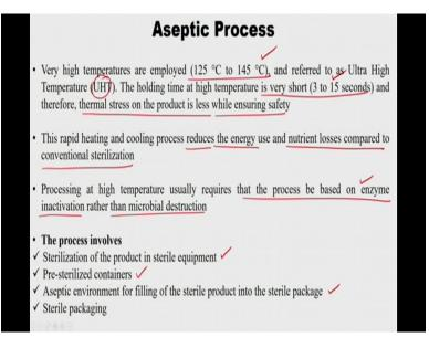
So the aseptic process is nothing but UHT. The very high temperatures are being employed almost 125 degree centigrade to 145 degree centigrade. So these are referred to ultra high temperature that is how it is called UHT. The holding time at high temperature is very short as I already told. If you keep it in very short time you can retain your nutritional qualities and also the thermal stress on the product is very less while ensuring the safety aspects as well. So this
