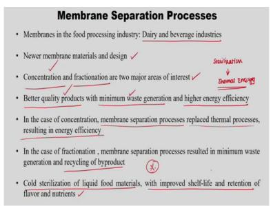
So, in the membrane separation process the major usage is in dairy as well as beverage industry. And, due to newer membrane materials and design so this field is very much useful in the food industries. And also the concentration and fractionation are two major areas of the interest in the membrane separation process. So, better quality products with minimum waste generation and higher energy efficiency would be the goal of the membrane separation process in food industry.
