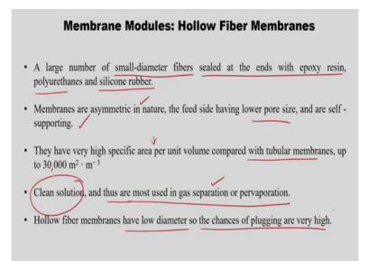
So, the next one is hallow fibre membranes a large number of small diameters fibres sealed at the ends with epoxy resin, polyurethanes as well as the silicon rubber. The membranes are asymmetric in nature, and feed side having lower pore size, and are self supporting. So, they have a very high specific area per unit volume. So, what are all the disadvantage of tubular membranes so that are taken care in the hallow fibre membrane and per unit volume compared with the tubular membrane.
