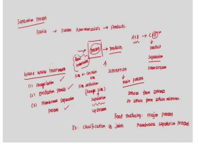
So, the first one we suppose to see is what is separation process and few basics about this. So, if any industry the main aim is to process raw materials and convert them into products. So, this is my process so I have a raw materials, so which are converted into products. But, so here my process requires my raw materials in some form. For example, so we take a size of
