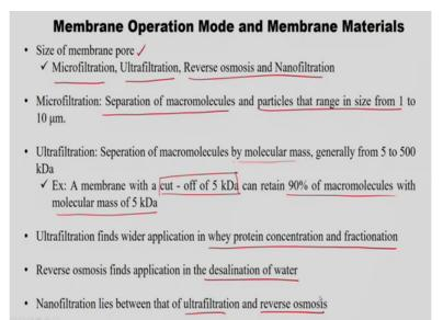
So, then membrane operation mode and membrane materials. The size of the membrane pores very much important. Based on that we will have variety of membrane separation processes as I told earlier microfiltration, ultrafiltration, reverse osmosis and nano-filtration. The microfiltration the separation of micro molecules and particles that range in size from 1 to 10 micro meter that is nothing but a microfiltration.
