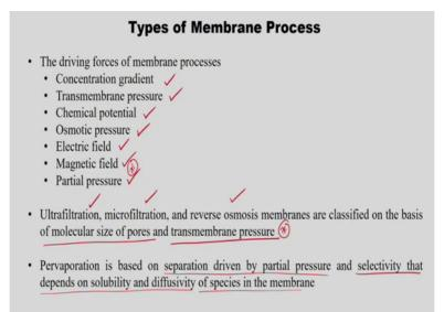
And the driving forces for membrane processes concentration gradient, transmembrane pressure, chemical potential, osmatic pressure, electric field, osmatic pressure in reverse osmosis, then transmembrane pressure and concentration gradient, magnetic field, partial pressure, so all of them are driving force based on the particular membrane separation process. So the major categories are ultrafiltration, microfiltration, and reverse osmosis. So,
