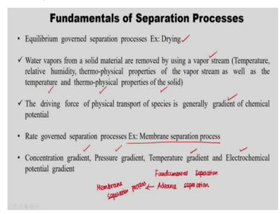
The equilibrium governed separation process are drying we just discussed. The water vapors from a solid material are removed by using a vapor stream. So, here the vapors stream the important parameters are temperature, relative humidity and thermos physical properties of the vapors stream as well as the temperature the physical properties of the solid is also important when we are doing the drying. Drying is nothing but a equilibrium governed separation process.
