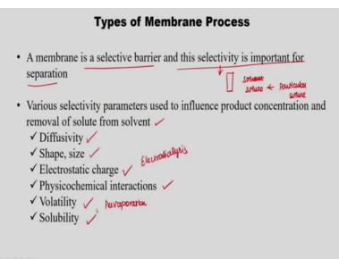
And, types of membrane processes so as we discuss few slides before. The membrane is selective barrier and this selectivity is important for separation. So, that means whether my membrane allows the solvent or solute or among the particular solute. Alright so based on this selectivity so we divide the processes and the various selectivity parameters used to influence the product concentration and removal of solute from the solvent. So, one is diffusivity size and shape of the particle.
