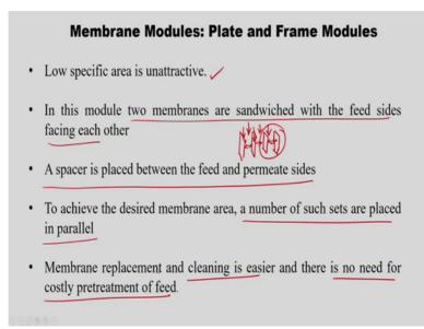
So, then next one is plate and frame module so here also low specific area which is also unattractive. In this module two membranes are sandwiched with the feed sides facing each other. So, that means so I have a membrane, so this is the feed side of this membrane, this is the feed side of this membrane. So, feed side facing each other it is tact, so that means the feed is going in between two. So, the permeate goes out of the membrane and retentate gets collected.
