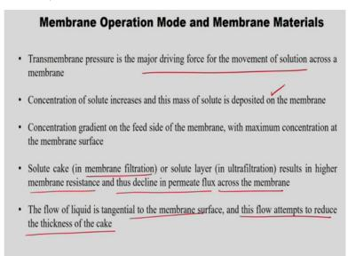
The transmembrane pressure is the major driving force for the movement of solution across the membrane. And, the concentration of solute increases at this mass of solute is deposited on the membrane surface we just discussed. The concentration gradient on the feed side of the membrane with maximum concentration at the membrane surface. So, maximum concentration happens at the membrane surface. And the solute cake or solute layer, solute cake in the sense in the case of membrane filtration.
