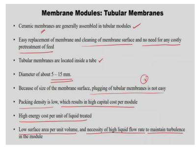
Now, we are going to see about the different modules, tubular hollow fibre membrane platen frame as well as the spiral wound module. The ceramic membranes are generally assembled in a tubular modules. If the material is membrane materials ceramic easy replacement of the membrane and cleaning of the membrane surface and no need for any costly pretreatment of the feed is the advantage of tubular membranes. Tubular membrane are located inside the tube and the diameter is about 5 to 15 millimetre.
