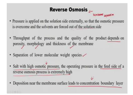
So, then another basic operation so, this also we are going to see in detail about them advanced membrane separation processes as well. So, here we will just see the basic definition and what happens in that reverse osmosis. So, the pressure is applied on the solution side externally so that the osmatic pressure is over comes and the solvents are forced out of the solution side. So, what we have done in the osmosis is, so from the solvent side the solvent moves to the solution side.
