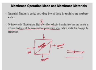
And the tangential filtration is carried out, where flow of liquid is parallel to the membrane. So as we said earlier so, this is my membrane process. So, where your feed is in here, so you will have the permeate, so then you will also have retentiate. Permeates is which passes through the membrane, retentiate is what gets retained in the membrane. The filtration is carried out were the flow feed is parallel to membrane.
