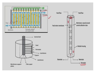
So, we are going to see here so this is your plate and frame modules, so if you see these are all membranes. So the feed is entered here so you will collect the retantate here and the permeate is getting collected from the membrane module here. So the feed as well as the retantate goes in the alternative compartment. So this is nothing but a spiral wound, so spiral wound your membrane is wrapped in the central line.
