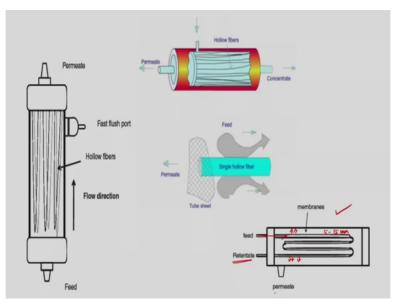
So, the next one is hollow fibre any we are having here so this is the tubular membrane. This is your tubes of 5 to 15 mm so here your feed is in. So, your permeate gets across the membrane and retentate will be retained and taken out, and the permeate comes out of the membrane and it gets collected in the tube module.
