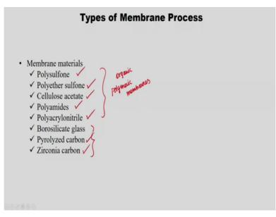
And membrane materials polysulfone, polyether sulfone and cellulose acetate polyamides and polyacrylonitrile. So, these are all polymeric membranes organic polymeric membranes. So, we also have the organic membranes which are nothing but a borosilicate glass, pyrolyzed carbon, zirconia carbon. So these are also widely used.
