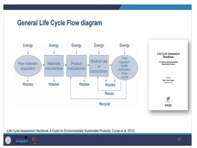
Here in this example, you can see the general lifecycle flow diagram. Here you can see, how the raw material is acquired, and even when the raw material is acquired, there is a certain consumption of energy and then at that stage itself, the waste is produced. Then, the material when is manufactured after acquiring the raw material, again the energy is consumed in the manufacturing process and then the waste is generated.
