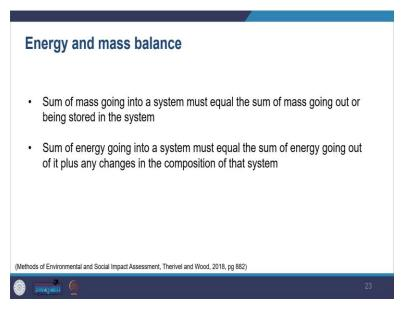
And when we talk about energy and mass balance, it means the sum of mass going into a system like the total energy getting into the system must be equal to what is coming out of the system. So, there should be a mass balance. And that sum of energy that goes into the system must equal the energy that is going out, plus the changes in the composition of that system.
