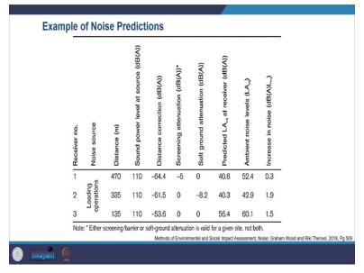
Here again, you can see different receiver numbers, 1, 2, and 3, and then the noise source and how far they are, what is the sound power level at the source, and then what is the distance corrections you are making. And then the screening, how the sound is reducing, what kind of soft surfaces are there, and then what is the predicted sound level at the receiver, and then what kind of ambient noise level is there, and what kind of what will be the increase in the noise.
