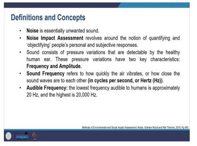
And then when we do undertake noise impact assessments, we look into quantifying and having a very objective understanding of how people are going to respond to that particular sound. So, we try to understand or when we say objectify that means having consistency across all the receivers and then giving a quantity of value to that response.
