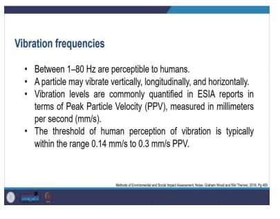
So, vibration frequency, frequencies between 1 to 80 hertz are perceptible to humans, we perceive that, and then the particle may vibrate vertically, longitudinally, and horizontally as well. And it is all, it involves, it often it is like a combination of all these three vertical, horizontal, longitudinal.
