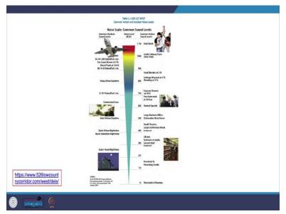
Also, here you can see common indoor and outdoor noise levels. You can see on the left-hand side all common outdoor sound levels and then common indoor sound levels, and then how, starting from the threshold of hearing at the bottom.
