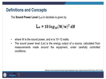
You can describe it as sound power where you indicate it by W, w and it is indicated as 10 to 12 watts. So, sound power level which is like L W is the energy output of a source. So, how much energy is coming out from
