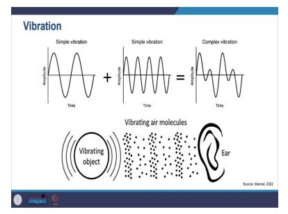
Now, look at the basic principle of vibration. So, what is vibration? Vibration is vibration refers to the oscillation of an object about a reference point. So, with like what kind, what number of oscillations per second is happening, and that is given in the form of frequency of vibration.
