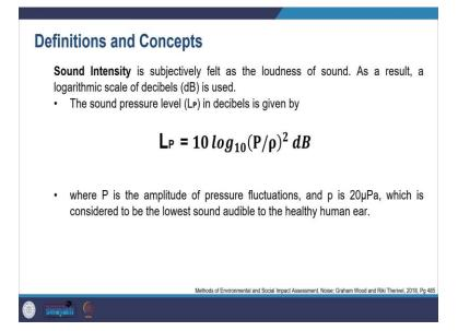
So, sound intensity is subjectively felt. So, it is like, it depends on the receiver. And it is like said as the loudness of the sound, how loud it is. And so it is indicated in the form of a logarithmic scale of decibels, you indicate in log decibel. That is how it is represented, sound intensity.
