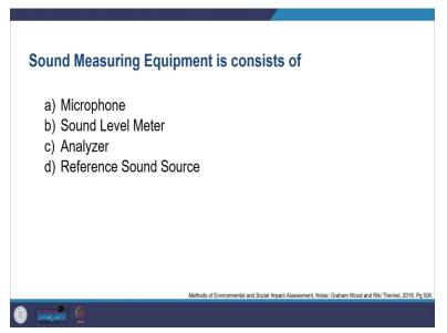
So, if you look at different kinds of equipment which are used for measuring the sound you have a microphone, which converts changes in ambient pressure into electrical quantity. And it is usually protected by the windshield. Then you have a sound level meter, which gives you information in dB. Then you have an analyzer, which records noise descriptors. So, you have LAeq, LA max, and so on over some time. So, they provide you with that.
