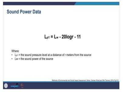
So, when you have sound power data, this is generally provided by the manufacturer, and you input data accordingly. So, here you can see the formula. So, it is a very basic calculation here, and what you see in 11 is like the correction that you make for the distance here. So, you have L p 1, the sound pressure level at a distance of r, from the source, and L w, the sound power of the source. And then 11 is taken as the correction factor.
