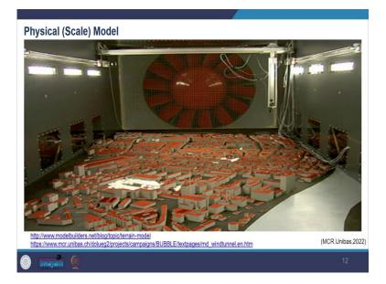
We see that, occasionally physical scale model is being used with a combination of wind tunnels and we also see the usage of computer graphics for impact prediction and evaluation. In particular, these are used in conditions where topography is complex, such as hilly terrain also when numerical models indicate uncertainty. So, whenever, you use a numerical model, it indicates a certain level of uncertainty regarding the pattern of effects due to the surrounding buildings and terrain.
