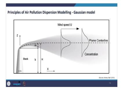
For example, in chimney stack, the basic Gaussian model considers that the pollutant emission spreads outward from a source in an expanding plume aligned to the wind direction. So, it goes in the wind direction it spreads in such a way that the distribution of pollution concentration decreases as the distance increases both in vertical distance or in horizontal distance. So, mostly the average shape of the plume is cone-shaped.
