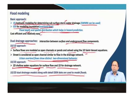
The basic approach is to consider the minor network that is the sewer network or the sub surface storm water drainage only. We use 1D hydraulic modeling for determining the sub surface storm water drainage and for this we can use the SWMM software that we have learnt earlier. We can use it for determining that how the water is actually travelling through a particular storm water channel. We can determine which are the nodes that are getting flooded.
