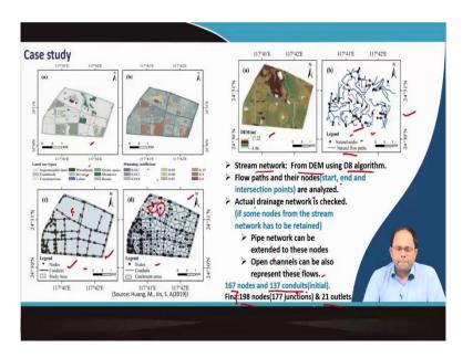
The land use type i.e., impermeable farmlands constructions woodlands rivers and the Manning's coefficient for each of these particular catchments were actually determined and once that is determined, then then based on the natural slope of that particular area or the DEM of that area, the natural flow channels were determined.
