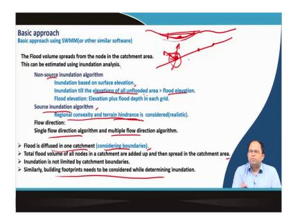
So, as we are discussing in the basic approach we assume the node flooding using SWMM and the flood volume spreads from the node in the catchment area and this can be estimated using inundation analysis. So, there are different forms of inundation algorithm.
