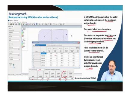
We can see that in SWMM flooding occurs when water surface at a node exceeds the maximum assigned depth of that particular node. So, we have already seen the node depths at every junction. The maximum depth is 0.3 feet and if it exceeds the ground level, then there would be flooding.
