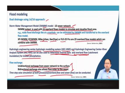
To do the 1D 2D approach, we use storm water management model for determining the flow in the sewer network. SWMM output is next used, that means, that node flooding data from SWMM is used with the 2D overland flow models to simulate and visualize flood area.
