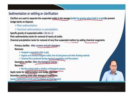
This step is exactly the same as in water treatment. *Plain sedimentation* (for all solids), and *chemical sedimentation or precipitation* (for removing fine suspended matter particularly colloids with the addition of chemical coagulants) are involved. Clarifiers are used to separate the suspended solids (with specific gravity 1.01 to 1.2 – is higher than that of water enabling settling) in the sewage which settles by gravity when held in a tank to prevent sludge banks on disposal.
