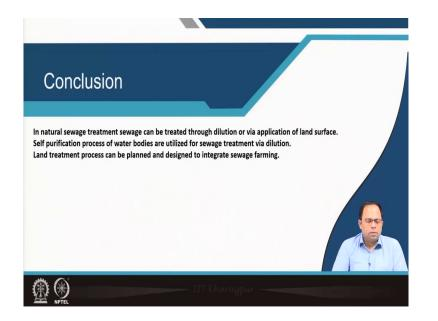
In natural sewage treatments, sewage can be treated through dilution or via the application on the land surfaces. The self-purification process of water bodies is utilized for sewage treatment via dilution. Land treatment process can be planned and designed to integrate sewage farming.
