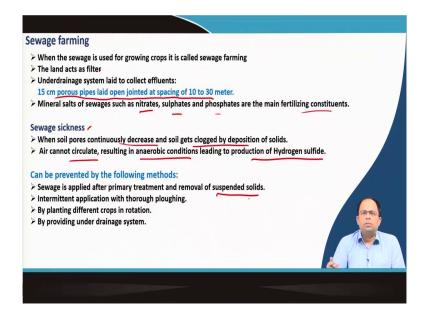
Sewage has the potential to become fertilizer for growing crops. Land act as a filter. The under drainage system is laid to collect the effluents (15 centimeter porous pipes are laid open jointed at a spacing of 10 to 30 meters) which conveys the percolated water to the disposal point. Mineral salts of sewage such as nitrates, sulphates, phosphates are the main fertilizing constituents that can help in the growth of vegetables or other crops.
