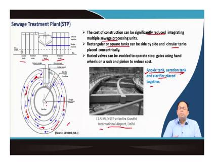
The case study shows the design of a 17.5 MLD sewage treatment plant at Indira Gandhi International Airport in Delhi. There is an anoxic tank, aeration tank and a clarifier placed together as a compact unit. In clarification tank, sludge is scrapped during sedimentation. In aeration tank, oxygen is added. In anoxic tank, nitrification happens in the absence of oxygen. These processes are combined together in one plant.
