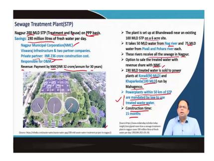
The case study shows the design of a 200 MLD sewage treatment plant in Nagpur. In this case, the treated wastewater is being reused. This was developed on PPP basis. This plant led to savings of 190 million litres of fresh water per day. This project was developed by Nagpur Municipal Corporation and the PPP model was implemented via Vishwa Raj Infrastructure and two partner companies which formed a special purpose vehicle.
