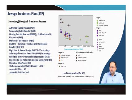
The Figure shows the land area required for an STP as per the different technologies as given in CPHEEO. These technologies are provided in combination. For example, a sewage treatment plant including trickling filter will require around 2500 square meter of area per million litres per day of sewage.
