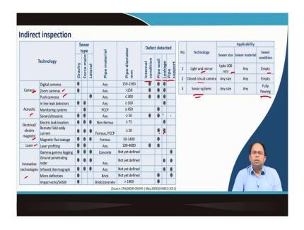
In indirect inspection, we use different kinds of technologies. The technologies could be use of digital camera, zoom cameras, push cameras in gravity sewers and for any kind of pipe (material, diameter) and the different kind of defects that could be detected are internal condition, pipe leakage, pipe support.
