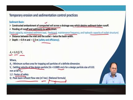
Sediment basin can also be designed. Sedimentation basin can be considered as a detention basin where we stop the water for a certain amount of time or allow ponding of water. This allows the sediment to settle for some time that can be dredged form the basin. Else, the sediment would be carried through the drainage channel. In this way it prevents erosion.
