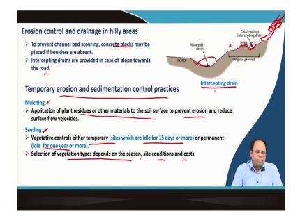
We can also provide intercepting drains. The water that is coming down the hill to a given channel carries lot of erosion. If the channel is blocked it will create floods.
