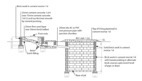
Pit should be raised by 300 mm (above water level during water logging)
