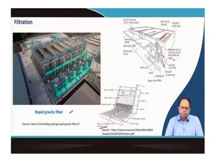
The Figure shows a rapid gravity filter. There are wash water troughs where water comes up and then it can be carried out through these troughs. It also shows the overall tank and pipelines, hydraulic valves etc. Drainage channels are also shown.
