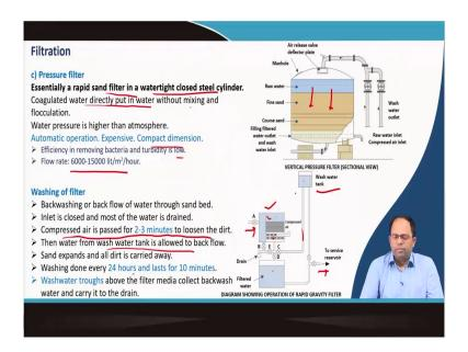
Pressure filter is another form of rapid gravity filter which is enclosed in a water tight closed steel cylinder. It is totally a compact process where coagulated water is directly put in without mixing and flocculation. The water pressure is higher than atmosphere as artificial pressure is created.
