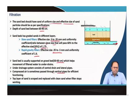
In sand filters, the sand beds should have sand of uniform size and effective size of sand particle should be as per specification. It has to be effective that means most of the sand has to be of particular size. Then depth of sand bed should be at least 60 to 90 centimeter.
