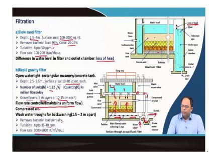
Regarding the design of slow sand filter, the water comes from sedimentation tank to the first chamber from where the water goes into the main filter. From here, the water goes down where fine sand is at the top, followed by coarse sand or pebbles or gravels. Below these layers, there is under drainage system from where water is collected into a sump which is taken out.
