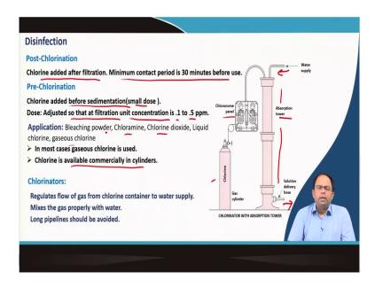
Usually there is pre-chlorination and post-chlorination. Post-chlorination is adding of chlorine after the process of filtration. Minimum contact period is 30 minutes before use.
