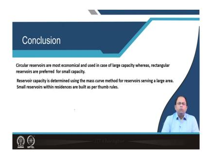
So, in conclusion we can say circular reservoirs are most economical and used in cases of large capacity. Whereas, rectangular reservoirs are preferred for small capacity. Reservoir capacity is determined using the mass curve method for reservoirs serving a large area. Small reservoirs within residences are built as per thumb rules.
