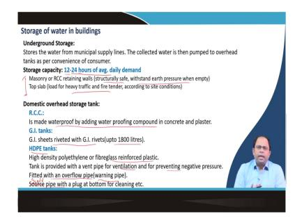
Underground storage in buildings stores the water from municipal supply lines. Whenever the water comes from the municipal lines, through ferrule, first, the water is collected in underground reservoir and then it is pumped to the overhead reservoir. If the pump is run twice then the reservoir capacity has to be for 12 hours and if it is run only once a day then the reservoir capacity has to be for 24 hours of average daily demand.
