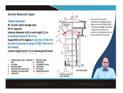
This is an example of a reinforced concrete circular water storage service reservoir. This particular reservoir is of 50 meter cube capacity. The internal diameter is around 4.65 meter and height of 3.3 meter and out of that 0.3 meter is the freeboard which is the top clearance. This is supported on reinforced concrete staging. There are 4 columns of 450 millimetre diameter with horizontal bracing of 300 to 450 mm at four levels.
