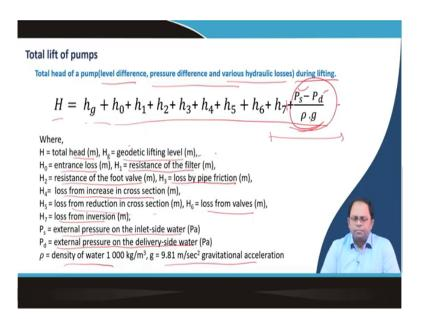
In addition to the standard suction lift, discharge lift and a head loss, there are other losses in the system because of presence of valves, entry pressure into the particular pipelines, etc. These can be ignored for broad calculations, but are needed for setting up pumping stations in various cases based on given situations.
