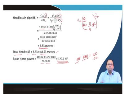
By applying Darcy Weisbach formula to calculate head loss in the pipe,
