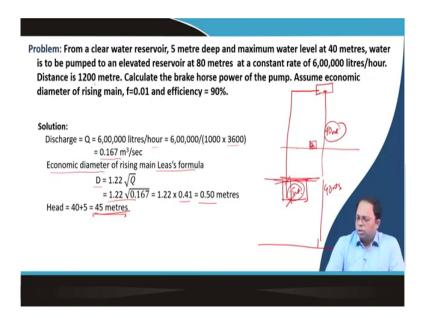
Problem: From a clear water reservoir, 5 metres deep and maximum water level at 40 metres, water is to be pumped to an elevated reservoir at 80 metres at a constant rate of 6,00,000 litres per hour. Distance is 1200 metres. Calculate the brake horse power of the pump. Assume economic diameter of the raising main, f = 0.01, and efficiency = 90%.
