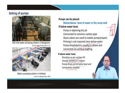
The above figure shows a 500 million litres per day water pumping station in Bangalore and a water pumping station in Kolkata. A large hall or structure houses several pumps which are aligned one after another and connected to one line.
