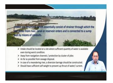
Intakes are structures which-<u>that</u> essentially consist of <u>a</u> strainer (similar to a screen) through which the raw water from the river, canal or reservoir enters and is connected to a <u>sump</u>, sump well <u>by means of using</u> conduits. <u>Strainer-The strainer</u> prevents the entry of impurities or big sized particles.\_-Sump stores the water before it is pumped into a treatment unit <u>or for other purposes</u>.
