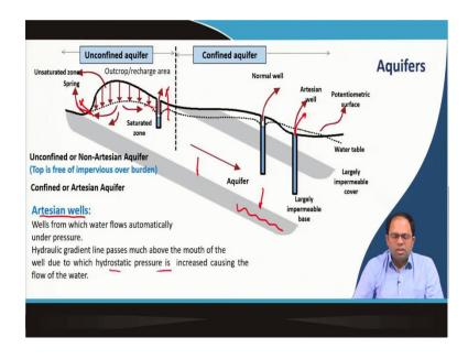
There are two types of aquifers; confined and unconfined aquifers. So, in this image you can see that the first part is unconfined aquifer and the second part is confined aquifer. The grey band is the impermeable base and water cannot flow beyond it. This is the water bearing stratum. Above this is the saturated zone, but we have got another impervious layer above as seen in the slide.
