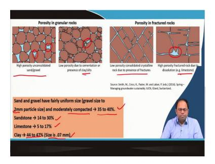
So, you can see over here that, this is sand and gravel. It is highly porous and these are unconsolidated and hence there are a lot of gaps in between the particles and these are of larger size. There is enough space for water to be stored. In the case of clay and silt, even though there are pores, porosity is low due to cementation or presence of clay silt.
