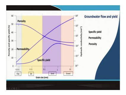
So, this is the graph which shows how for different particles or different kinds of soil, like clay, silt, sand and gravel these 3 parameters vary; porosity, permeability and specific yield.
