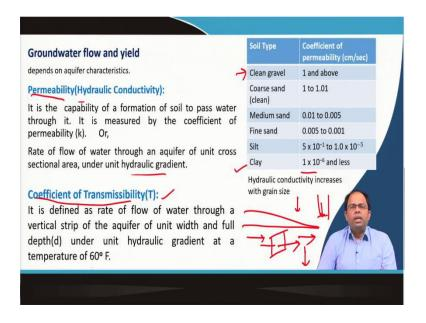
Next we look into two aquifer properties or characteristics of the aquifer, this is known as permeability which is also known as the hydraulic conductivity and the other is coefficient of transmissibility.
