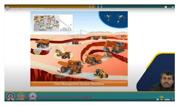
FMS workflow: FMS system for a mine site, is a set of software running on rugged hardware. Using GPS and a wireless radio network, the FMS tracks and monitors production maintenance and safety in the mine. At the top, we have the control center connected to the wireless network and a GPS satellite network. The wireless network sends a signal to equipment that is fitted with an onboard computer. The equipment sends
