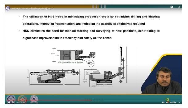
Let us discuss the autonomous drill rigs. We will start with an example of the Epiroc smartROC D65. The smart ROC D65 incorporates cutting-edge automation technology to facilitate drilling in various scenarios, including production blast, pre-split, and buffer holes. The drill offers a reverse circulation option for in-pit grade control as well. The
