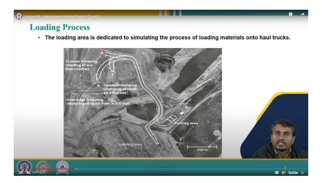
into the crusher. Second is over-edge dumping, dumping of earthen materials from the cliff top, and third is the paddock of dumping, dumping of earthen material on the flat side. There is another side that is a parking area where the vehicles will park during their ideal time or maybe during their maintenance time. So, this is basically the route map for testing the configurations.
