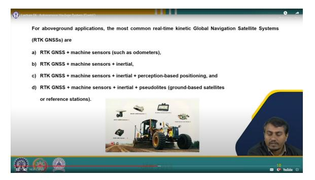
So, this is basically the machine having all these facilities to get an accurate position. Here is the inertial measurement unit, here is the GPS antenna, here is the GPS receiver, here is the control system, and here is the hydraulic valve model. So, these are basically fitted onto this machine and everything working in tandem so that machine can perform
