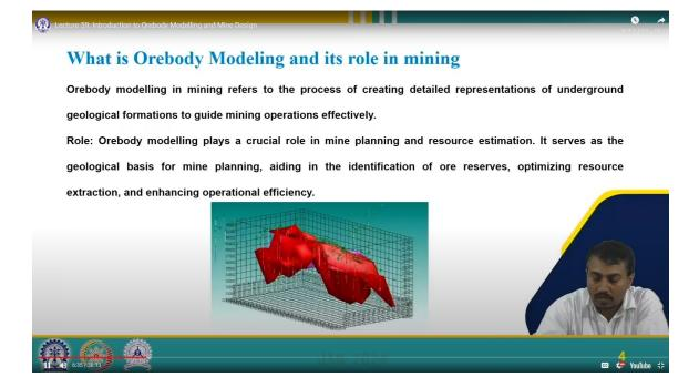
So what is ore body modeling and its role in mining? So, if you look into this figure, this particular figure represents a kind of interpolation based on some data points and its
