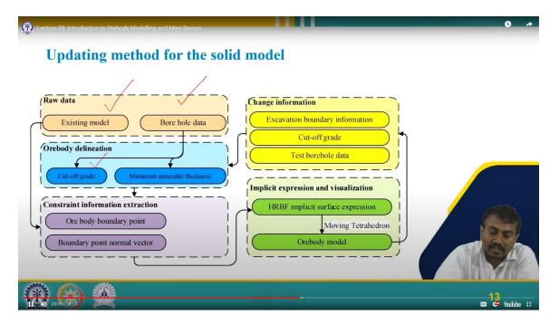
So, step number one is the ore body delineation according to the cut-off grade, and the minimum mineable thickness of the ore body boundary is determined. Step number two is the extraction of ore body boundary control information. The ore body boundary
