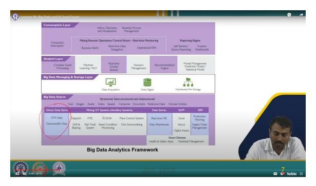
So, this particular picture shows, in a graph, the main framework of data analytics in mining. So here you can see the direct data stores, GPS data, and operational technology that operate in mining: FMS, SCADA, Real Track system, drill and blast, dispatch, plant control system, ore geo modeling, and asset condition monitoring. The data stores, real-time database, data warehouse, format, Excel, Word, digital assets, ERP, and other
