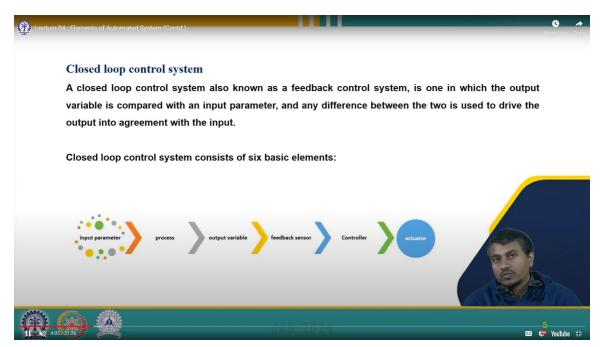
Input parameter: The input parameter, often referred to as the set point, represents the desired value of the output. So, this is a very important point here because based on this value and the output value, it will compare, and based on that, the closed loop system basically reruns the system.
