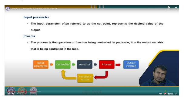
Output variable: The output variable is some process variable, perhaps a critical performance measure in the process such as temperature, force, or flow rate. A sensor is used to measure the output variable and close the loop between input and output. Sensors perform the feedback function in a closed-loop control system.
