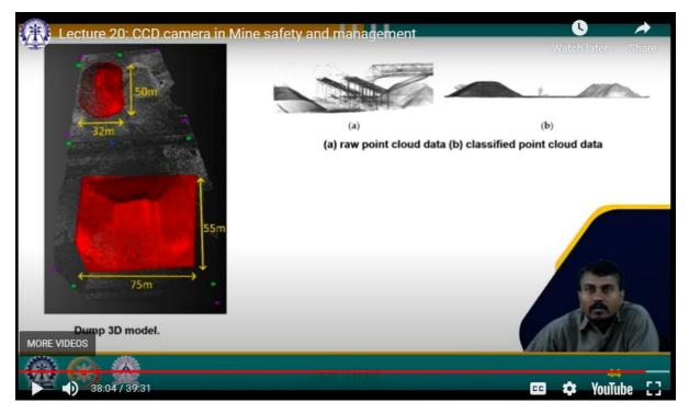
Point cloud and excavation site before and after video recording. So, we can assess easily how much activity is going on, so we can develop using this image some index of activity going on in that particular site.
