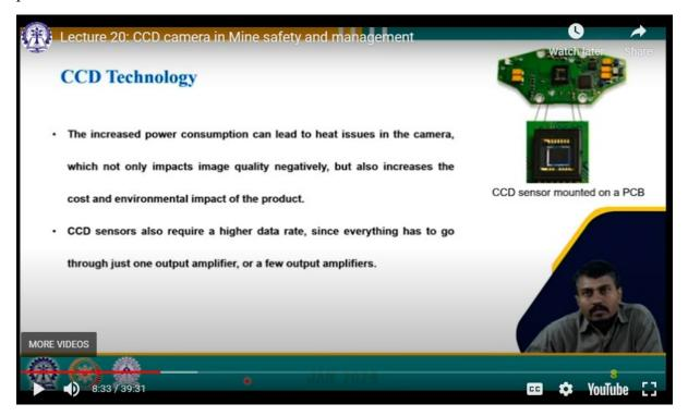
The basic operation in CCD technology. In a CCD for capturing images there is a photo active regions okay a layer of silicon and a transmission region made out of a shift register that is we have already explained the few slides back with the horizontal shift register and the vertical
