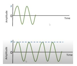
If we compare these two pulses, the one in the bottom being have more cycles compared to the one in the top, they have the same pressure amplitudes, but the one in the bottom will have more acoustic energy. And the way we would measure the pressure amplitude would be based on this practical setup.
