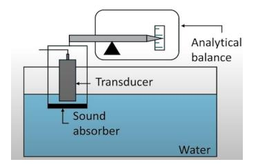
So, this is what radiation force is. We can use this radiation force balance here. So, this is a schematic of what experimental setup using a radiation force balance looks like. We have our transducer here that is then sending an ultrasound field towards a sound absorber right here. So, this will be the target. And this sound absorber is connected to an analytical balance that you can use to measure the force.
