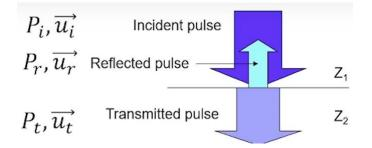
Now the particle velocities are vectors, so there's a directional dependence on them. And when we compute the reflection coefficient, we are actually computing the fraction of the incident pulse that is actually being sent towards the pressure of the reflected pulse.
