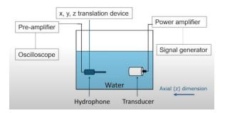
So, what we had here is a setup that consists of a hydrophone, which is used to measure acoustic pressure distributions, as well as the shape of the ultrasound beam. Now this hydrophone, you can think of it as a microphone for ultrasonic frequencies, and this hydrophone can be immersed.
