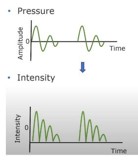
This is just a schematic example. And a couple of intensity metrics that you can calculate are first being the temporal peak intensity, or  $I_{TP}$ , which is the peak intensity at that instant when the pulse peaks. Now, this is the maximum value of the intensity within that pulse. And then we can also calculate I\_PA, which is much lower than the temporal peak intensity.  $I_{PA}$  corresponds to the pulse average intensity.
