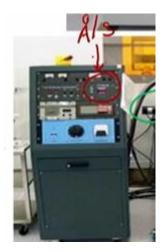
Then there is a variac. And a current meter to show the current in terms of amperes. There is also a vacuum pump and another control electronics right.
