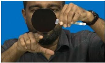
This is a primary flat on top and there is secondary flat in the bottom. So, if there is secondary flat with respect to primary flat at 180 degree it is N type 100.
