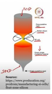
A melt zone is established between lower seed material and upper feed material. This is done by heating it the feed material when it comes in contact with the seed material using the radio frequency coil. The floating zone is moved along the rod that means, this will move along the rod in such a way that the crystal grows on the seed. So, that this will keeps on melting and this keeps on fabricating like growing.
