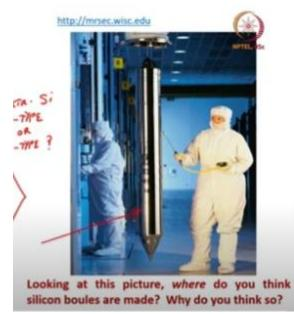
Why is all this gowning required? This is called personal protective equipment and also called the clean room gowns. So, the long cylinder you see there is a silicon boule and then the engineer is wearing all the PPEs and and checking the silicon boule. The question is, where do you think silicon boule are made? So, the answer would be that it should be in a clean room or foundry environment.
