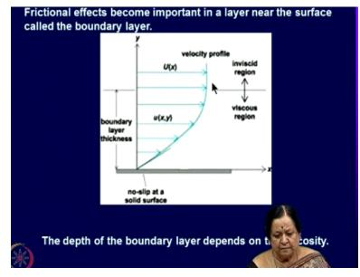
If you have a plate here and you have a flow like this okay this is the wind if you wish and this is the surface of the flat plate, then add the surface of the earth surely the air cannot go past it the there cannot be a slip so the boundary condition here is of no slip okay and frictional effects become important in a layer near the surface called a boundary layer and the whole purpose of the boundary layer is to satisfy the conditions at the surface of no slip.
