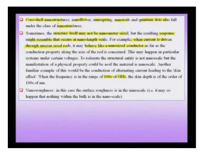
Like for instance suppose, I am driving through a normal conductor, alternating current when I am if I suppose, keep on increasing the frequency, then we know that even when alternating current is not carried throughout the conductor, most of the current density is in the outer region of the conductor which is called the skin of the conductor.
