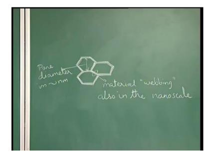
So, let me draw this in a little expanded fashion in the board. So, I have approximately hexagonal pores, and this pore diameter, it is pore diameter in the Nano scale, but actually it inter connects between the two, like this regime.
