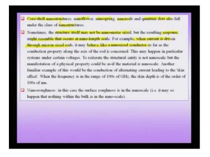
An interesting point to be noted here, we talk about also in the coming slides is the fact that, the structure itself may not be nano-meter sized, important class and it is very different. Now, we are not talking about a Nano structure in the classical sense of the word, that the scale of the structure is not in the Nano scale, but the response of the material, to a certain kind of stimulus could actually be occurring in the Nano scale.
