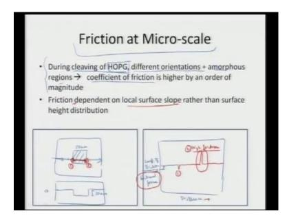
So, seeing the friction at micro skill we can see that once we can cleave the highly oriented pyrolytic graphite, we can see or because of different orientation. Which are present on a surface or because of amorphous region in the HOPG that is highly oriented pyrolytic graphite. What can happen is the coefficient of friction can alter to a certain extent.
