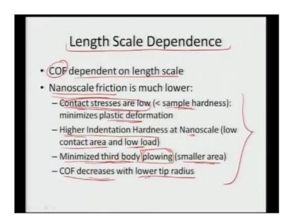
Also is dependence of coefficient of friction on the length scales, so coefficient for friction depends on the length scale as well what is happening what has been observed is that nano scale friction is much lower than that of the micron scale friction. And that is basically results because the contact stresses are very low.
