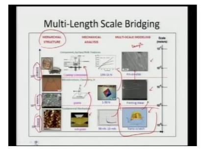
So, essentially what is happening is we have to correlate what is happening at nano scale micro scale and the macro scale. So, a kind of testing that is required, so at sub grain we are talking about nano indentation or nano scratching at micro scale we are talking about fretting and at macro scale we are talking about pin on disc. So, how we can correlate
