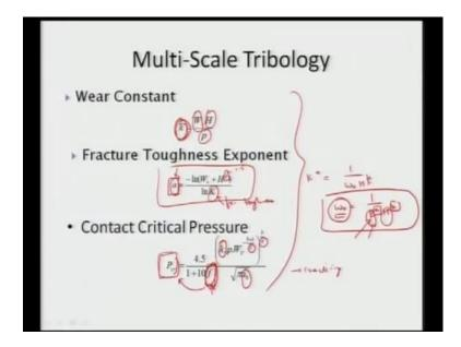
But, more essential is to be able to correlate what is happening at nano scale and at micron scale. So, we can see that the overall wear constant is dependent on the wear volume hardness of the material and the kind of loading that has been applied. So, we can obtain the wear constant and equating that. So, because we can also find the what is the fracture toughness for a brittle material when do see what is the crack length or what is the fracture toughness exponent.
